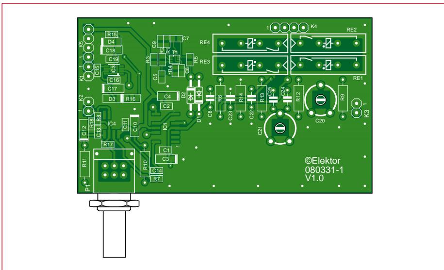
Figure 3. Printed circuit board for the amplifier.
